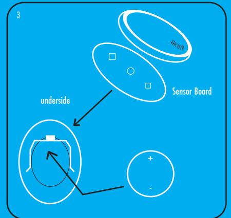
EN: Battery placed on underside of device board. Providing power to the unit.
