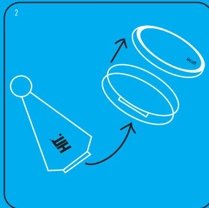
EN: To open Device use a finger nail to prise device seal apart. If you find this difficult use the small edge on the Magnet keyring to do this.
