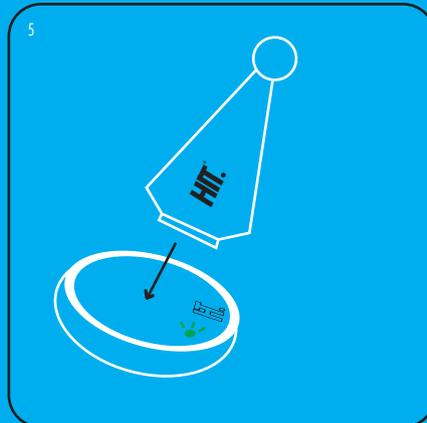
EN: To turn on device, Tap the magnet to the screen of the IMPACT device. A quicker tap is more efficient in opening the switch. The device will flash **GREEN** to confirm ready state.
