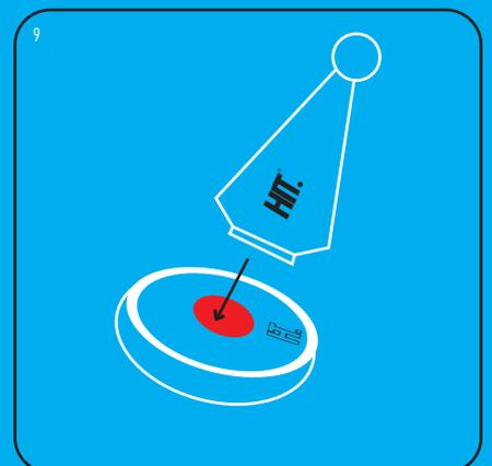
EN: To reset device after **RED** light or to turn off device simply tap with magnet again and all lights will turn off. Your device is now in off state. To turn back on to continue playing simply follow from step 5.
